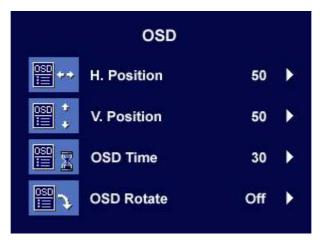
Press ◀ or ▶ key to adjust the Horizontal Position of the OSD, press "Exit" to return to previous menu.
